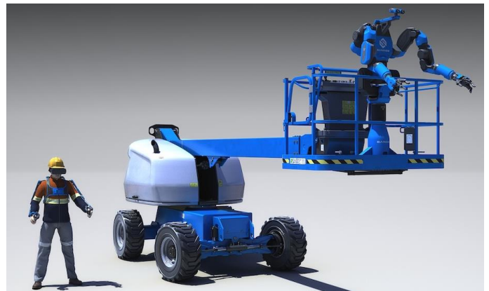
Figure 52 Guardian XT Teleoperated Dexterous Robot
