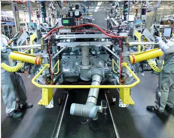
Figure 43 UR Cobot Used For Screwdriving In Auto Assembly Line
