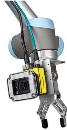
Figure 44 UR Cobot With An Integrated Cognex Camera
