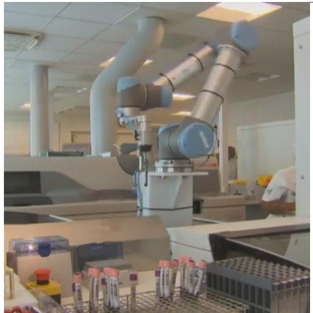
Figure 45 – A Cobot Used In A Lab For Testing Blood Samples
