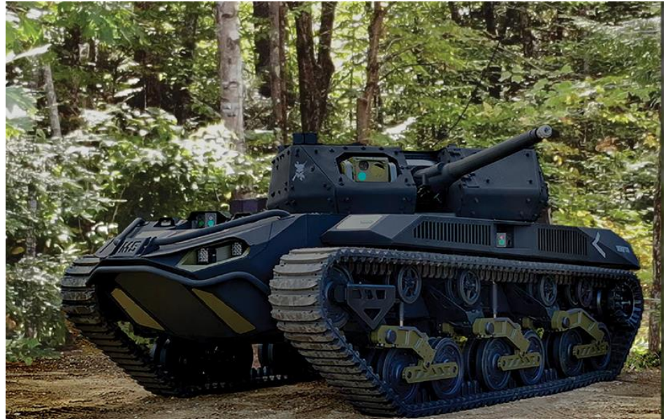
Figure 22 Robotic Combat Vehicle – Medium (Textron)
