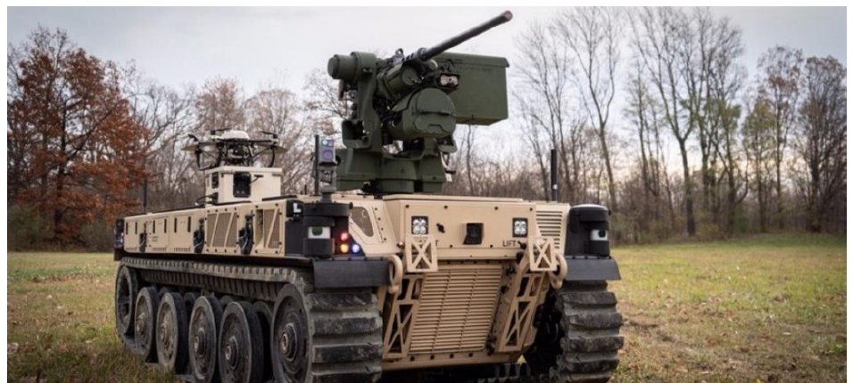
Figure 23 Robotic Combat Vehicle – Light (QinetiQ/Oshkosh-Pratt Miller)
