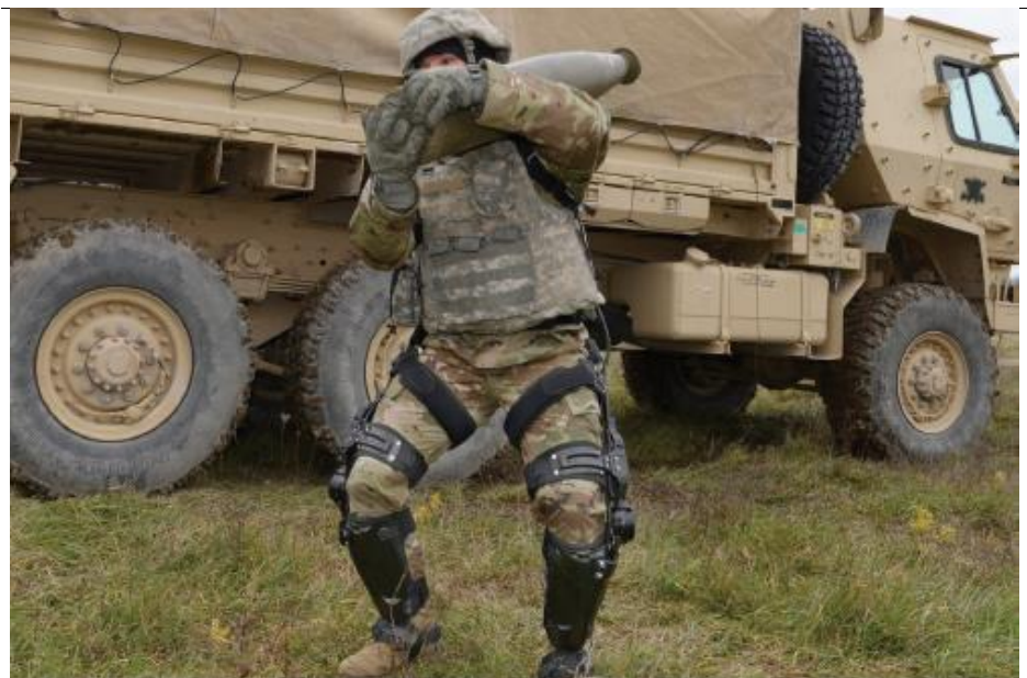
Figure 29 Lockheed Martin ONYX Lower Body Exoskeleton
