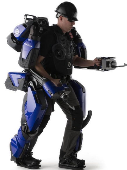
Figure 20 Sarcos Robotics Guardian XO Exoskeleton
