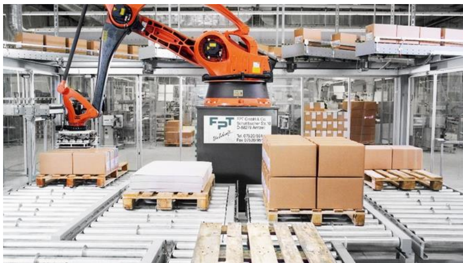
Figure 40 A KUKA Palletizing Robot
