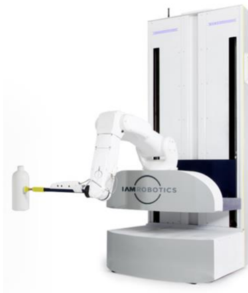
Figure 37 IAM Robotics AMMR For Autonomous Picking
