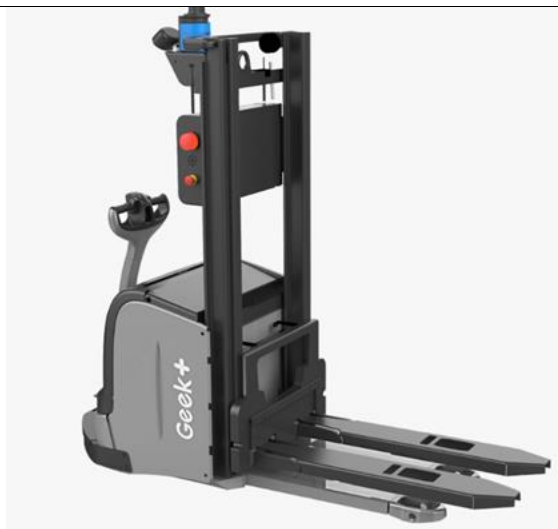
Figure 38 Geek+ Autonomous Forklift
