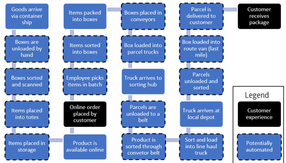
Figure 3 Various Steps That Make Up The Fulfillment Process Can Potentially Be Automated
