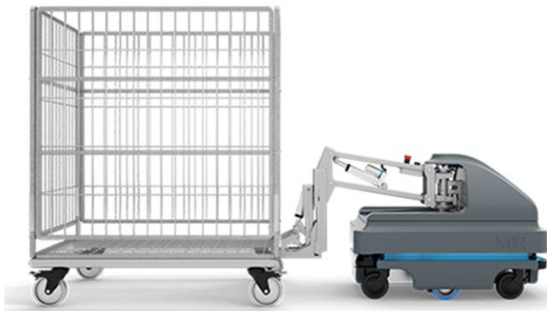
Figure 39 MiR Robot Utilized For Materials Transportation Within A Manufacturing Warehouse
